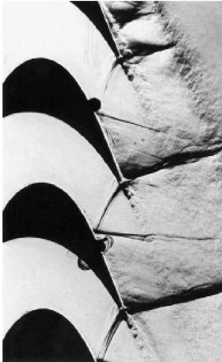
Schlieren photograph of flow in a highly loaded transonic turbine cascade with an exit Mach number of 1.15.
