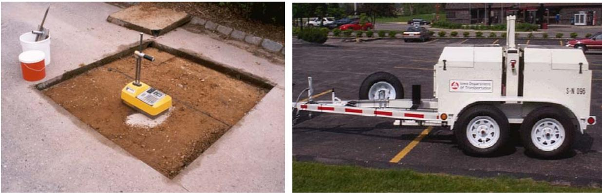
**Figure 9 Field density and Falling Weight Deflectometer Measurement**
