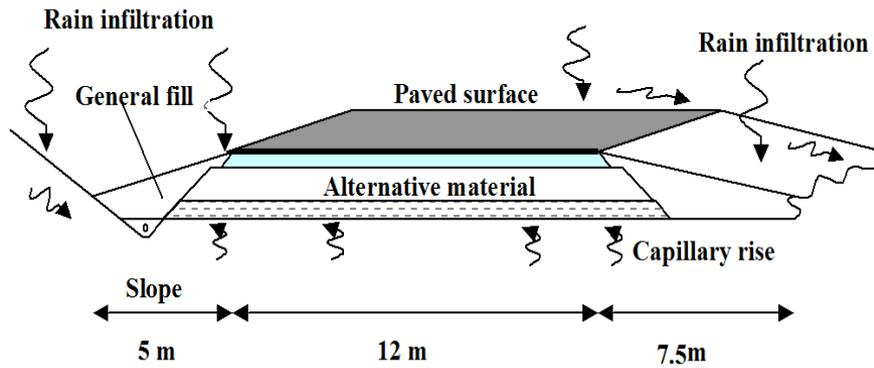
Figure 6 Water movement into a road infrastructures (source ALTMAT)
