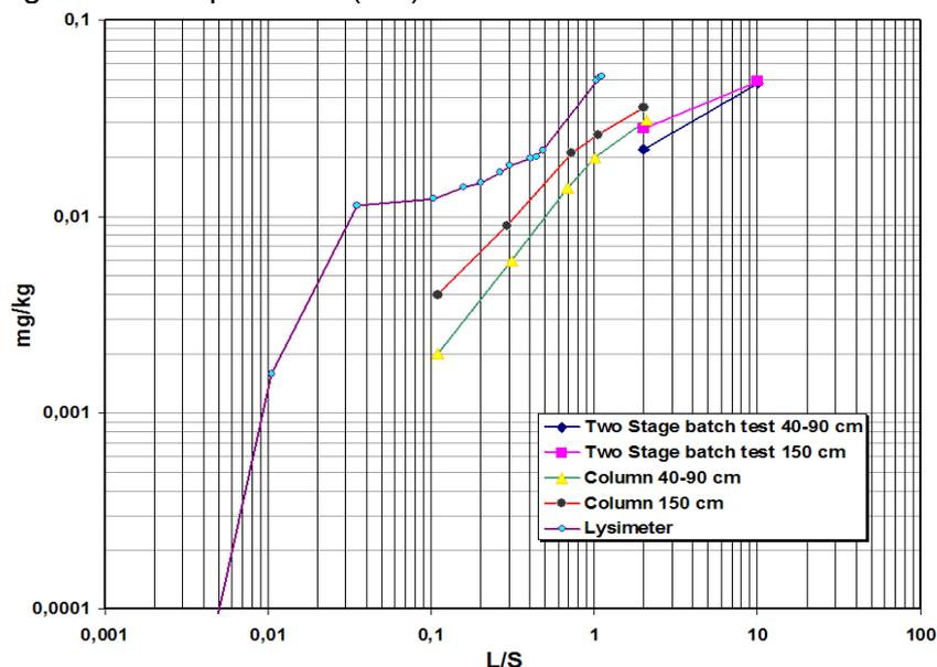
Figure 5 Amount leached (mg/kg) versus Liquid/Solid (L/S) ratio (source ALTMAT)
