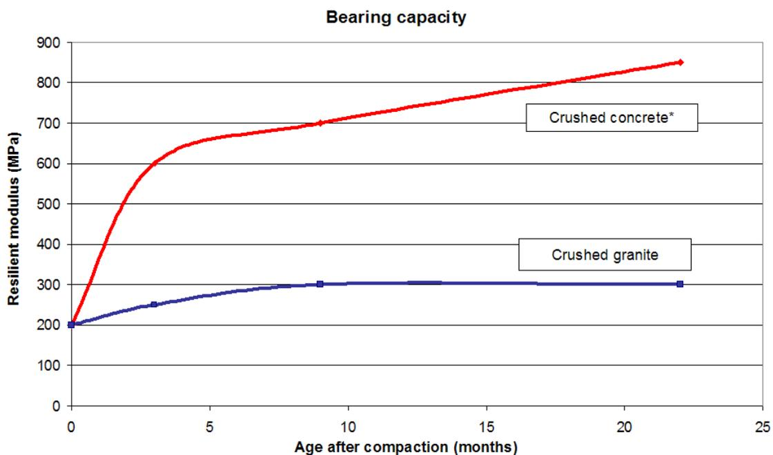
**Figure 8 Resilient modulus from FWD versus time for crushed concrete sub-base (source ALTMAT)**
