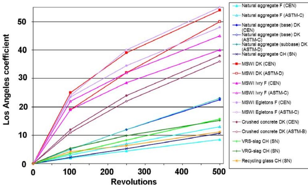
Figure 4 Los Angeles abrasion tests for alternative materials carried out under ALTMAT research program
