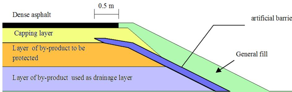
Figure 7 Mitigation by impermeable layers.
