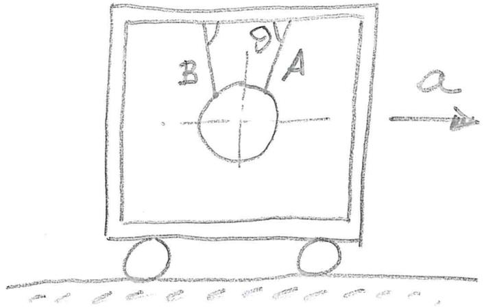
$$\left\{ \begin{array}{l} T_A \cos \vartheta - T_B \cos \vartheta - ma = 0 \\ T_A \sin \vartheta + T_B \sin \vartheta - mg = 0 \\ T_A = 2T_B \end{array} \right.$$
