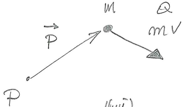
$$\begin{aligned} \frac{d\vec{K}_0}{dt} &= \frac{d\vec{P}}{dt} \wedge (m\vec{v}) + P \wedge \frac{d(m\vec{v})}{dt} = \vec{v} \wedge (m\vec{v}) + P \wedge \frac{d(m\vec{v})}{dt} = \\ &= \vec{P} \wedge m \frac{d\vec{v}}{dt} = \vec{P} \wedge m \vec{a} = \vec{P} \wedge \sum \vec{F}_e = \vec{M}_0 \end{aligned}$$
