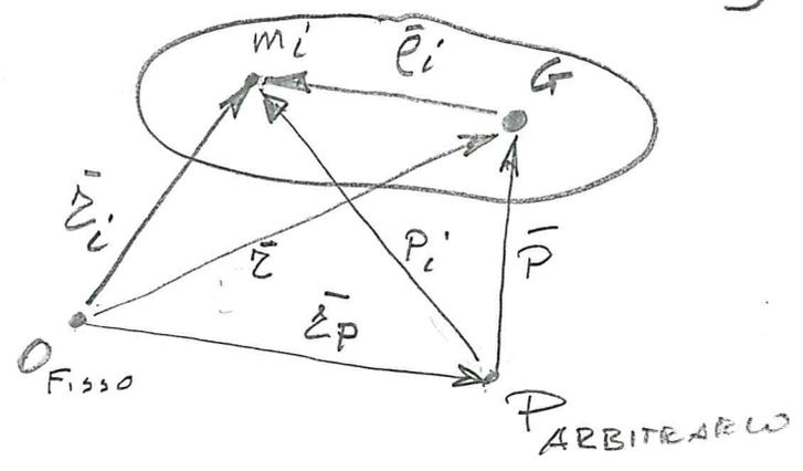
$$\begin{aligned} \bar{K}_P &= \sum \bar{P}_i \wedge m_i \bar{V}_i \\ &= \sum \bar{P}_i \wedge m_i \dot{\bar{r}}_i \end{aligned}$$
