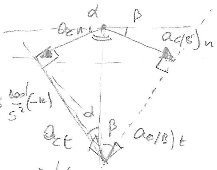
$$\omega_1 = \frac{a_{c/t}}{AC} = 1,73 \frac{\text{rad}}{\text{s}^2} (-\omega)$$
