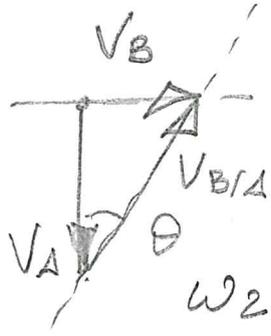
$\omega_2 = \frac{V_{B/A}}{AB} = 11,55 \frac{\text{rad}}{\text{s}} (-\vec{k})$
