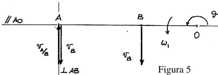
$$\vec{v}_{A/B} = -\vec{v}_B \Rightarrow \omega_2 = \frac{1}{l} v_{A/B} = 40 \text{ rad/s}$$
